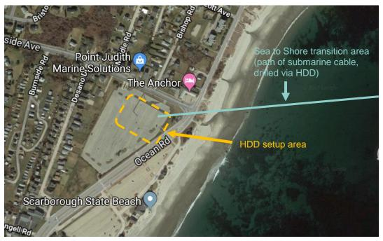
An HDD operation similar to that proposed for the South Fork Wind Farm was used successfully to install a submarine power cable at Scarborough Beach in Rhode Island. This process is different from the method used to install the submarine cables at Block Island and will set the cable to a much greater depth.
